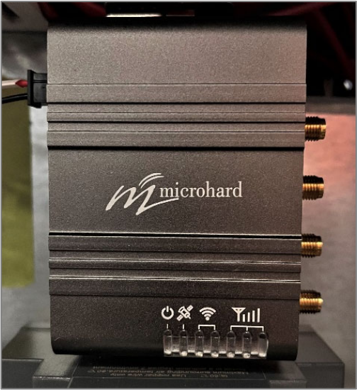
Figure 7-1 – Cellular Modem Located in the Electrical Enclosure
